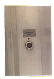
By using a 14mm box spanner, unscrew the nut underneath the thermal trip reset label from the inside of the still at Step 01
