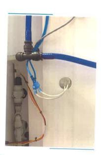
Connect the new thermal cut-out cables with the blue cables that you have just disconnected. Slide the thermal cut-out into the glass boiler, flat
